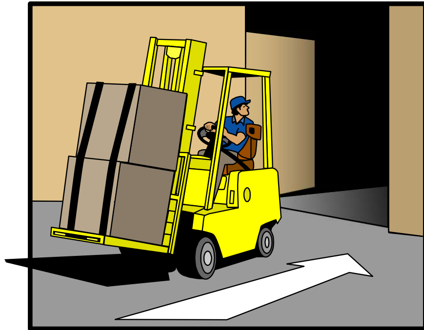
Drive Backwards with Load
